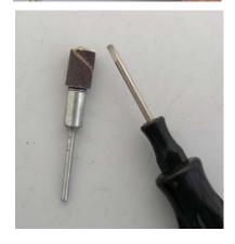
6. Mount the drum mandrel on a rotary tool and grind the copper flush with the bronze.
