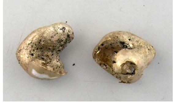
Copper clay was inlayed in fired silver hollow forms so that the copper surface was flush with the silver surface. The metals alloyed and the pieces melted.
