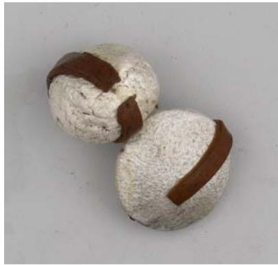
There was no alloying but the copper strip shrank and broke at the seam.
