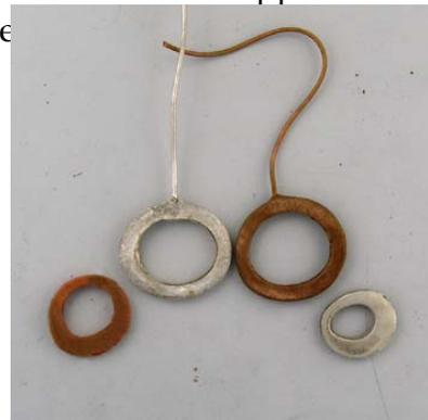
Copper washer was wrapped around silver washer; silver washer was wrapped around copper washer In both cases the silver and copper sintered but separated with very little effort.
