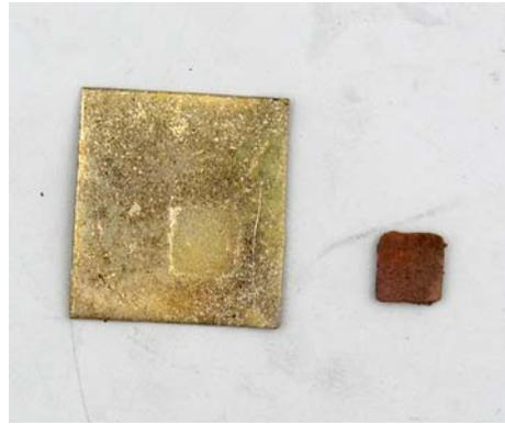
This experiment was done with sterling and fine silver sheet as well. An unfired square of copper clay was connected to fine silver sheet with oiled paste. The copper sintered but the pieces did not adhere.
