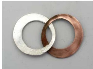
A silver washer and a copper washer were linked and fired with no contact between them. Both sintered well.
