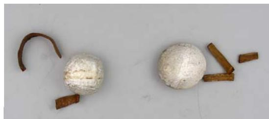
The strips broke easily to multiple pieces. They were not properly sintered.
