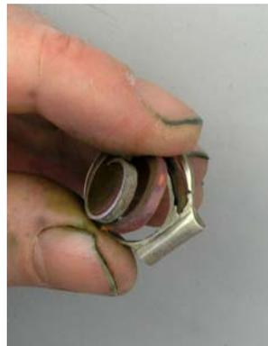
Here a strip of copper clay was placed on a strip of low-shrinkage silver clay and the two strips were rolled into a coil. The silver and the copper sintered, but easily separated.
